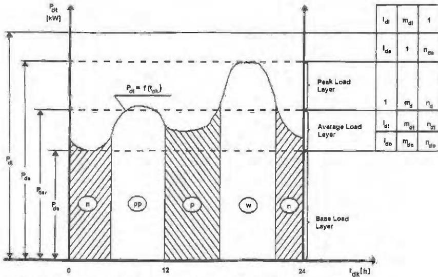
Fig. 4.1. The 24-hour load profile: the division into the layers and columns.
