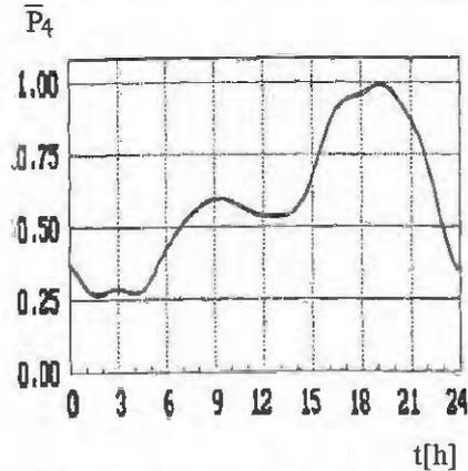
Fig.-4.4. Typical 24-hour load profile for class 4 customers (municipal-living)
